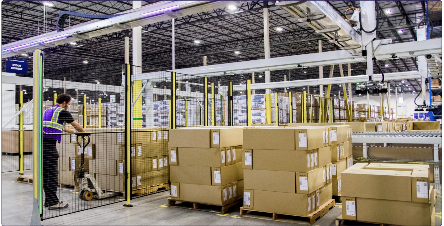
*Robot Operator entering safety zone to remove a complete pallet, while AmbiStack continues stacking to other zone
